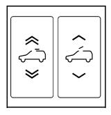
There are two switches in the overhead console that operate the sunroof.
